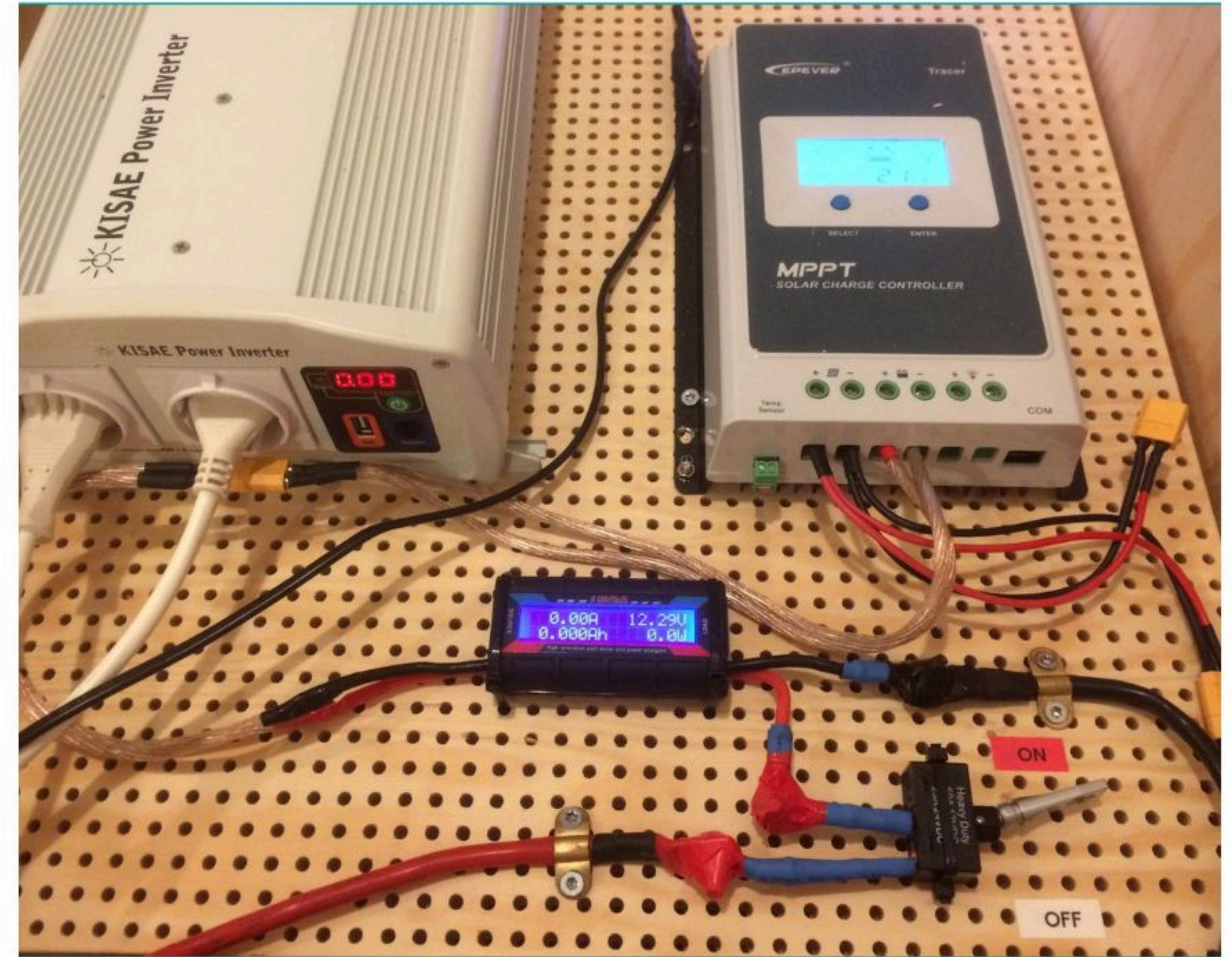
Inverter & charge controller
