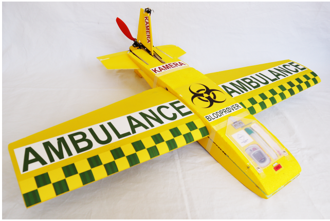
Fig. 1. Prototype blood sample transportation drone (photo by the authors)
