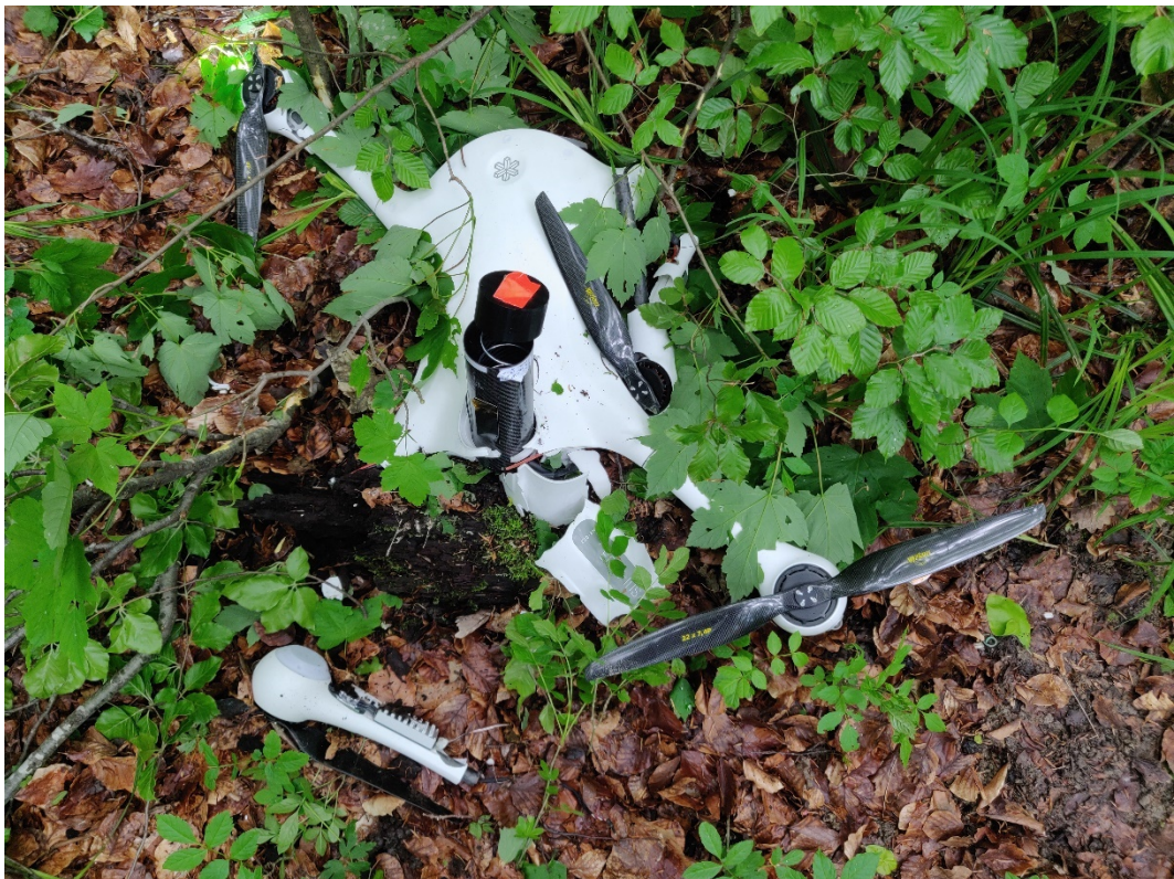
Figure 1: The Matternet (Matternet, 2021) drone which crashed in a wooded area of Switzerland near a kindergarten. The emergency parachute had been deployed, but the chord connecting it to the drone was cut allowing the 12 kg drone to freefall to the ground. Image used with permission, from (SUST, 2019).
