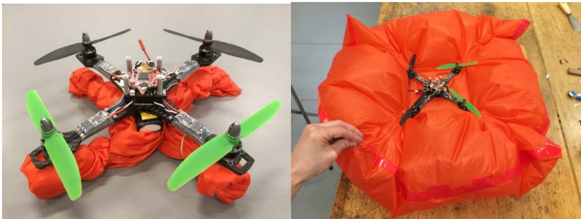
Figure 16 Airbag prototype number one; this prototype was made with standard parachute material. Experiments showed the airbag material did not hold air, and deflated quickly. It could be folded under the drone such that the drone could still fly.
