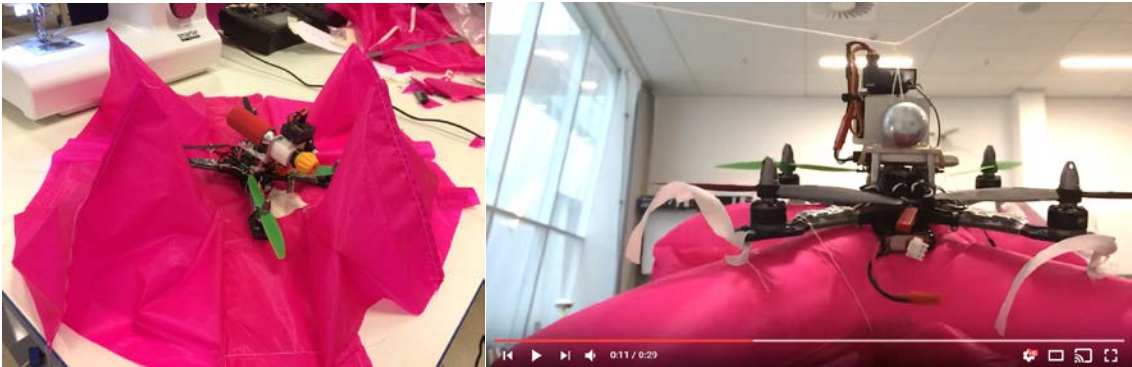
Figure 18 Airbag prototype number three; this prototype was X-shaped to follow the arms of the drone. It had a smaller volume to facilitate inflation and an inner bladder plastic welded at the seams (in practice the seams leaked when pressurized). The triangular-shaped drag flaps can be seen standing upright between the drone’s arms. An inflation test we carried out in the lab, then the system was field-tested.
