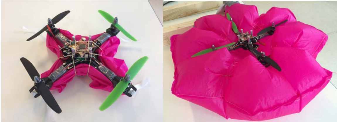
Figure 17 Airbag prototype number two; this prototype was constructed of zero-porosity parachute material. It showed it was possible to fabricate a robust airbag by sewing, but this induced leaks in the seams. The shape did not fully wrap around the drone as intended (only marginally). The shape did fold down tightly enough that the drone could still fly. This airbag was also used to check aerodynamic stability. It was filled with small styrofoam spheres (as it was not airtight), and dropped from two heights - 4 meters and 7 meters, at different orientations (bottom down, sideways, upside down, and thrown with spin). The airbag always landed bottom down, except when dropped upside down; then, it remained upside down.
