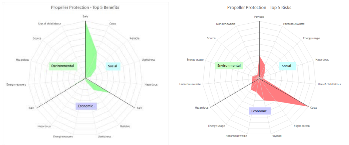
Figure 11 Radar chart output of the product assessment for propeller protection. Results are on a scale from zero to ten, zero being no impact and ten being high impact. Developed from: (B. University, 2016)
