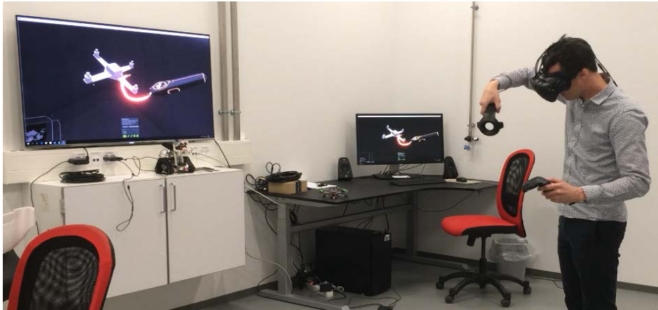
Figure 9 A CAD model of the drone was imported into a VR environment to allow airbags to be 'sketched' around it in three dimensions.
