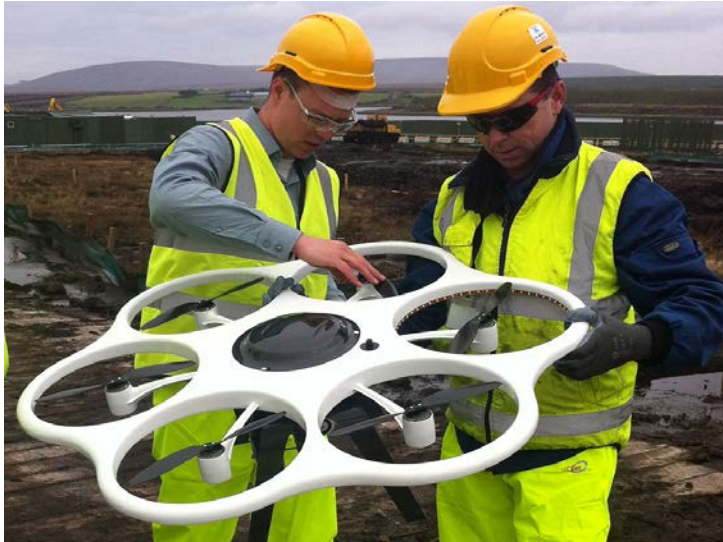
Figure 2 The Aibot X6 incorporates safety bumpers around the propellers as it is used for inspection and is frequently operated in close proximity to structures (X6, 2016).
