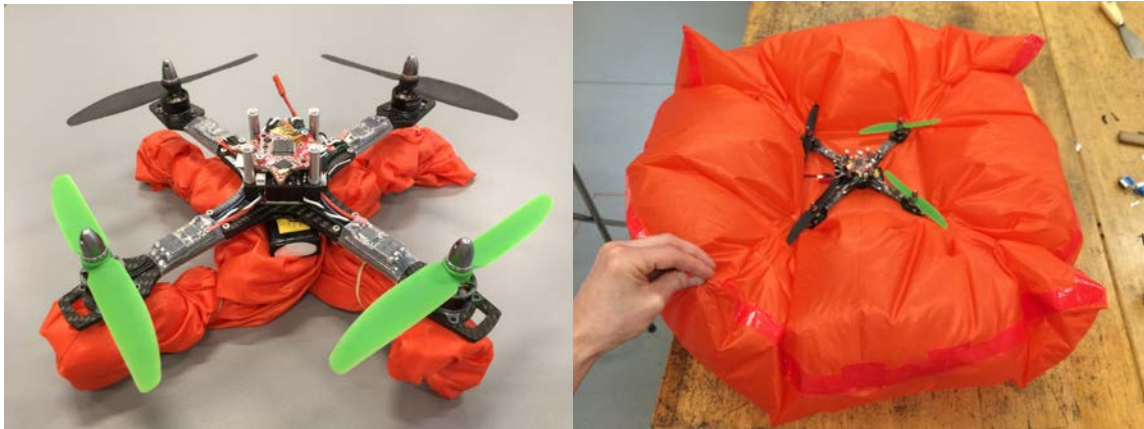
Figure 16 Airbag prototype number one; this prototype was made with standard parachute material. Experiments showed the airbag material did not hold air, and deflated quickly. It could be folded under the drone such that the drone could still fly.
