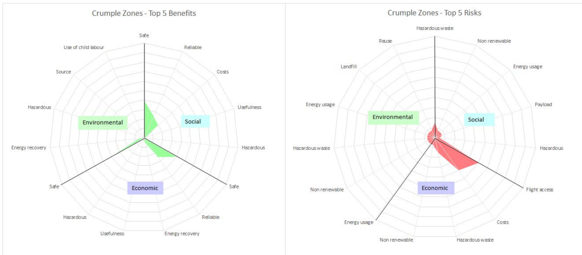
Figure 12 Radar chart output of the product assessment for crumple zones and foam padding. Results are on a scale from zero to ten, zero being no impact and ten being high impact. Developed from: (B. University, 2016)
