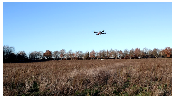
Fig. 7. The drone being tested in-situ; the drone was hovered for around 20 seconds at an altitude of approximately three meters and at a distance of about three meters from the test equipment. Image by the authors.
