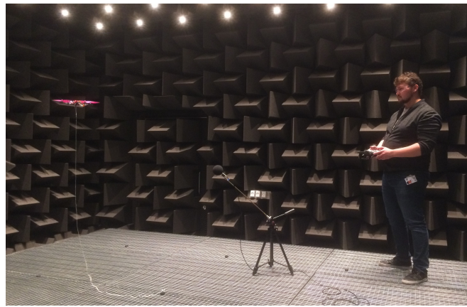
Fig. 8. The drone (left) being tested in the anechoic chamber; the drone was hovered in manual mode by the drone pilot (right) for around 60 seconds at distance of one meter from the test equipment. A B&K 4189 free-field microphone (center) was used. A string was tied to the drone and bolted to the grid floor to prevent the drone from damaging the walls of the chamber. Image by the authors, with consent granted by the subject in the image.
