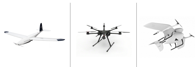
Fig. 1. Three types of smaller drones under 25 kg: a fixed-wing drone (left) [7], a multirotor drone (center) [8], and a hybrid vertical takeoff and landing (VTOL) drone (right) [9].
