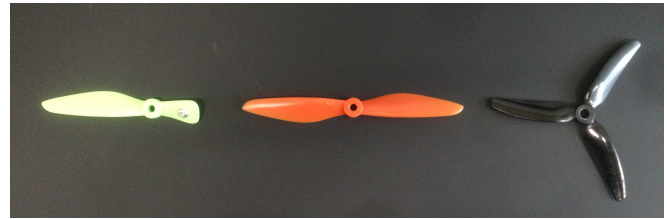
Fig. 6. The three propellers tested with one (left), two (center), and three blades (right). Image by the authors.
